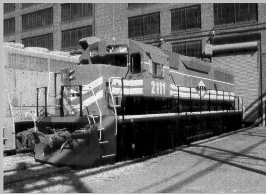
One of the first units of an anticipated 11 slug-slug mother sets for the Paducah and Louisville Railway. This is slug mother 2111 - a GP40 seen on April 27, 2001 at the VMV shops in Paducah.
